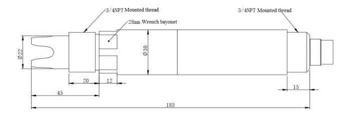
Note: The sensor connector is m16-5 core waterproof connector male.
