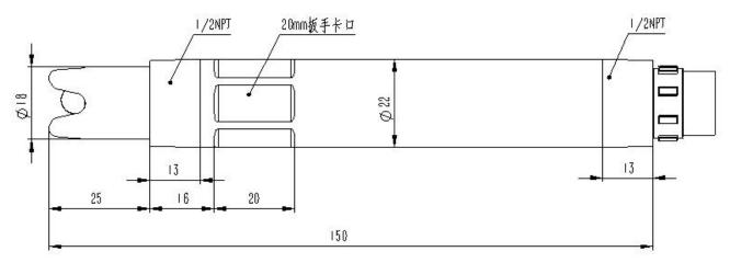
Note: The sensor connector is m16-5 core waterproof connector male.
