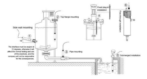
Note: The sensor should not be installed upside down or horizontally when installed, at least at an angle of 15 degrees or more.
