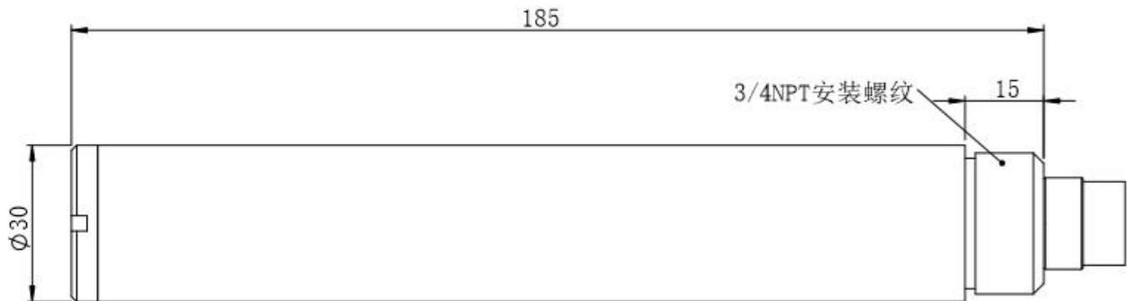
Note: The sensor connector is m16-5 core waterproof connector male.
