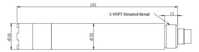
**Note:**The sensor connector is m16-5 core waterproof connector male.
