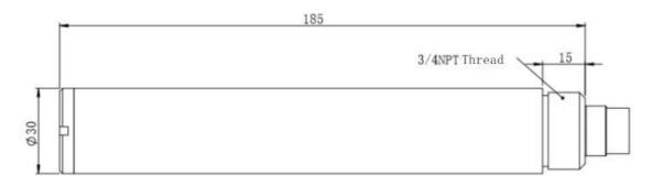
Note: The sensor connector is the male end of M16-5 core waterproof connector.
