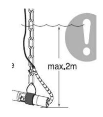
The sensor is placed in a position where there are no bubbles in the water.
