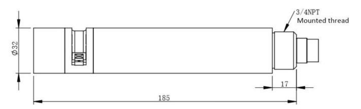
Note: The sensor connector is a male M16-5 core waterproof connector
