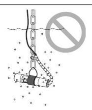
Note: It is recommended to install a cable protective cover on the outside of the sensor cable. The sensor can be placed in any direction in the water. It is recommended that the sensor be placed horizontally and firmly fixed, and the measuring area should face the direction of the water flow.
