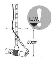
Install the sensor to a depth of no more than 2 meters from the water surface.
