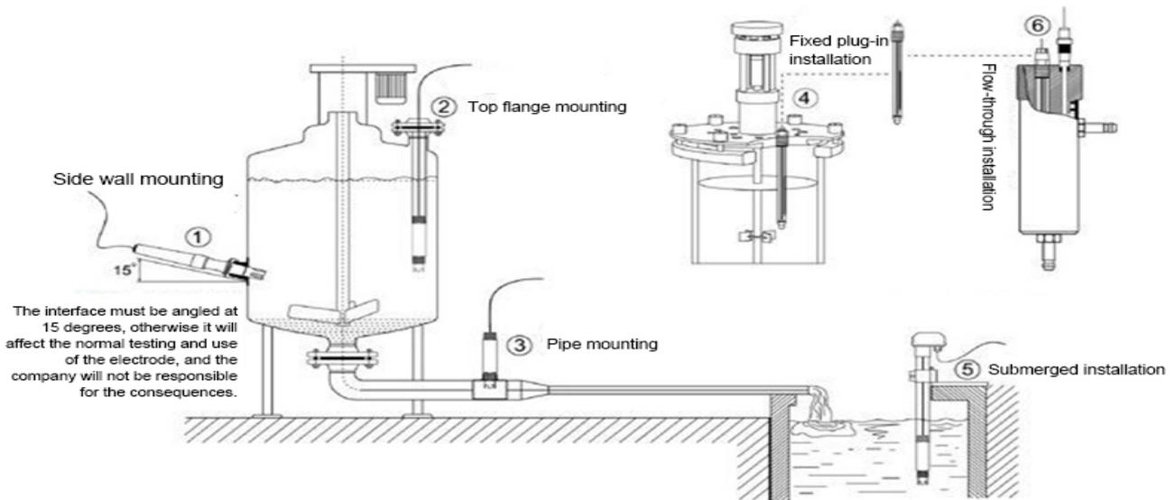
Note: At least 2 cm from the bottom and side walls of the container during installing and testing.
