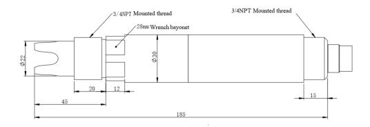
Note: The sensor connector is M16-5 core waterproof joint male head.
