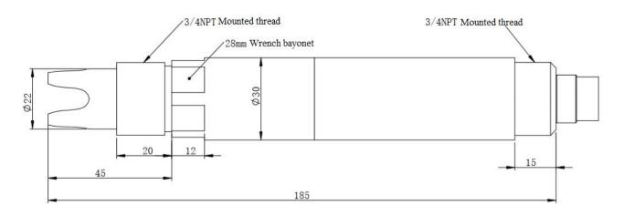
Note: The sensor connector is m16-5 core waterproof connector male.
