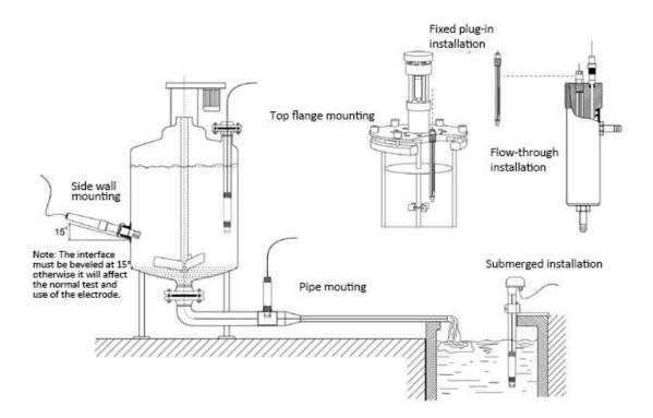
Note: When the sensor is installed, it cannot be installed upside down or horizontally, and it must be installed at an angle of at least 15 degrees.
